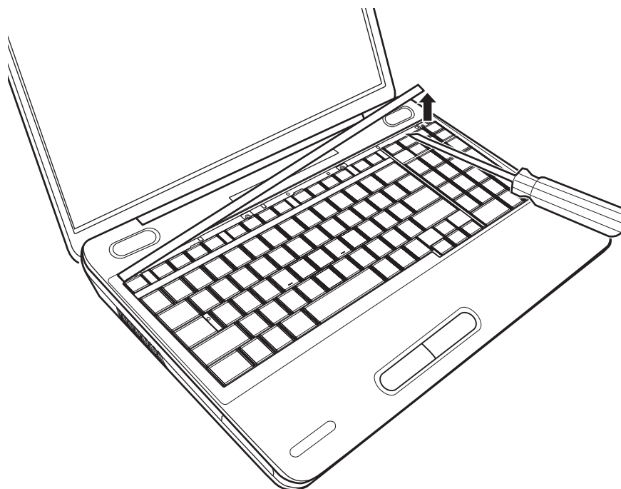
Figure 4.8 Removing the keyboard cover
